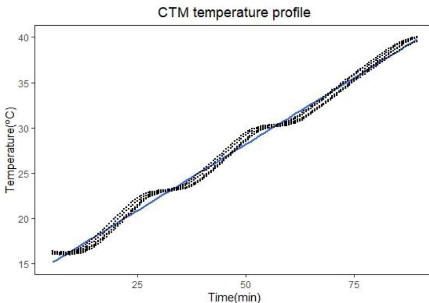
Fig. 2. Critical Thermal Maximum temperature profile achieved using a PID controller with a temperature increase of  $0.28^{\circ}\text{C}$  per minute.
