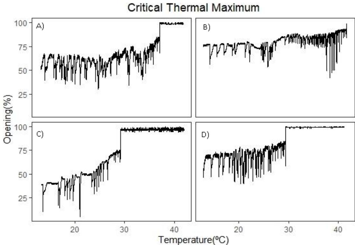
Fig. 3. Valvometry of *Unio tumidus* (A and B) and *Anodonta anatina* (C and D) to the critical thermal maximum. The valve movement is represented as opening percentage.
